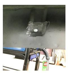
**6.** Using the battery box insert as a guide, mark the four mounting holes in the trunk floor and drill these holes out using a 25/64-inch drill bit.
