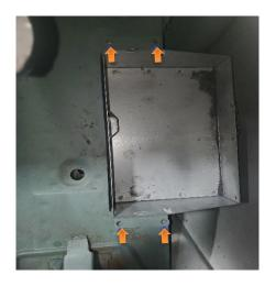
**8.** Using the center stamping depression of the trunk drop-off panel as a guide, measure down three inches and mark the spot for drilling.
