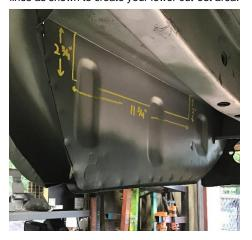
3. With all cut lines marked proceed to cut the marked metal area out using the cutting method of your choice. Plasma cutter or cutoff wheel work great for the confines of the area. Once the metal has been cut free, grind/file any rough edges.
