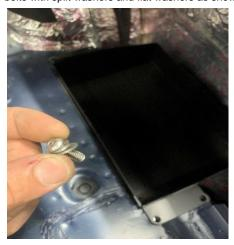
17. Install the fasteners assembled in step 16. Hand start all four fasteners to ensure proper alignment of the battery box and to prevent cross threading the fasteners. Tighten the fasteners evenly to secure the battery box in place.
