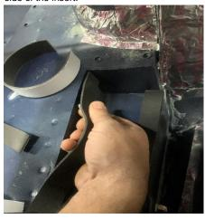
**14.** Insert the battery vent hose grommet into the hole just drilled. Then pass the vent hose through the grommet to the underside of the battery tray and secure it to the vehicle, leaving enough hose to reach the battery once installed.
