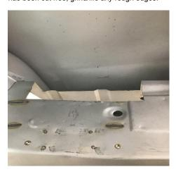
**4.** Place the insert into the cutout opening and check for proper fit. File/grind the opening as necessary to provide the proper fit for welding. Prep the area and the insert for welding by scuffing all areas to clean and remove old paint and other contaminants and then fully weld the insert into place.
