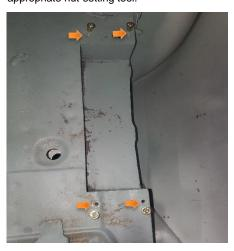
**09.** Drill the marked spot out with a 3/8-inch drill bit, deburr the hole, and grind or sand the metal bare as shown.
