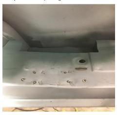
**7.** Locate the supplied nut inserts and install them into the four holes just created using the appropriate nut-setting tool.
