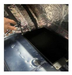
**18.** Insert the hold down clamp J-hooks into the slots found in the battery box side panels, place your battery into the tray, and secure with the hold-down clamp and J-hooks using the included hardware. Connect the battery positive and negative cables to the battery and secure the battery vent hose to the battery.
