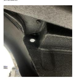
**15.** Using the 3/8-inch external star washer, 3/8-inch flat washer, and the 3/8-24 nut, install the battery ground cable to the stud welded in earlier.
