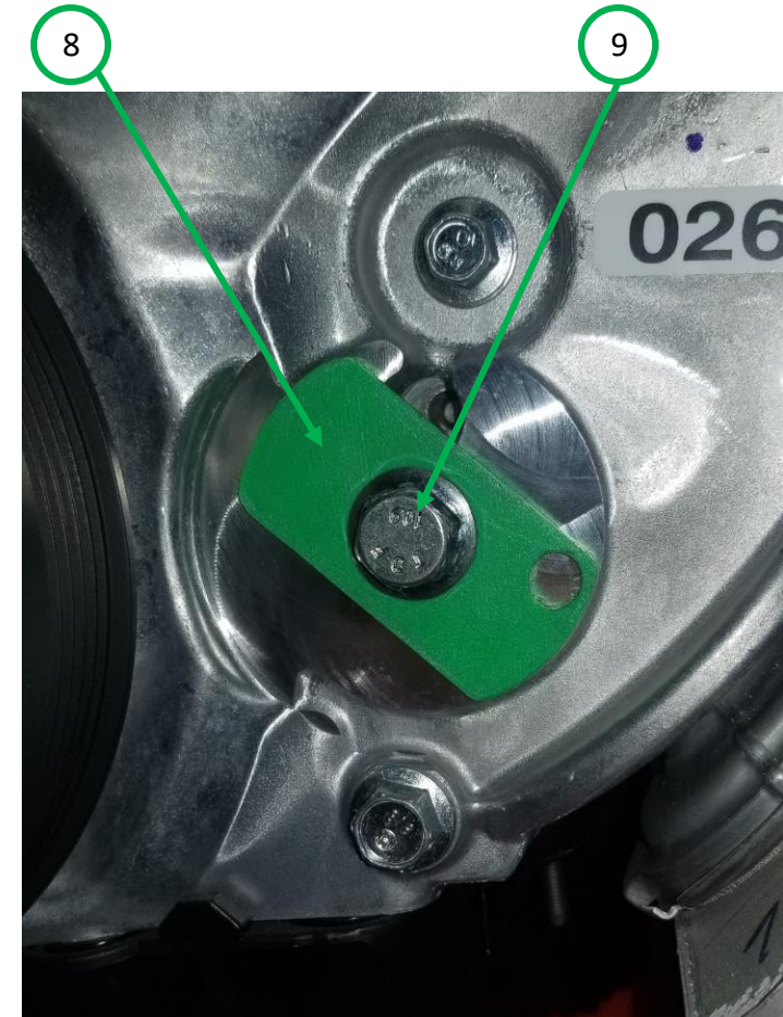
TIGHTEN TENSIONER CLOCKING TOOL TO ENGINE. USE 17/64" DRILL BIT TO CREATE NEW TENSIONER CLOCKING HOLE. DRILL TO A DEPTH OF 3/8".
