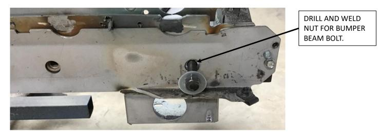
WELD BUMPER BEAM NUT FROM INSIDE AFTER ALIGNING WITH BOLT.
