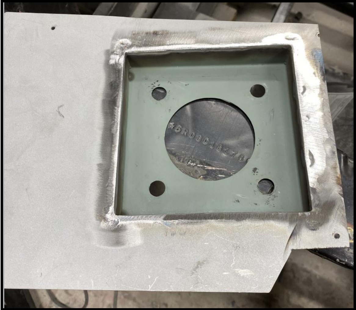
CLEAN UP WELDED EDGES (1966 FIREWALL PLATE SHOWN SAME PROCEDURE FOR 1967-1968 FIREWALL PLATE)
