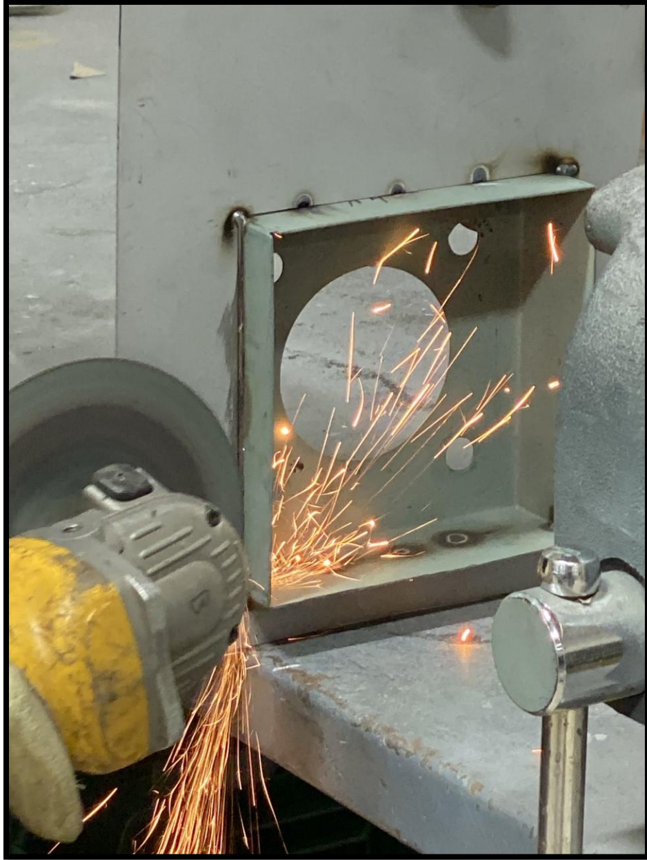
TRIM EXCESS FLANGE HANGING OUTSIDE OF PLATE
