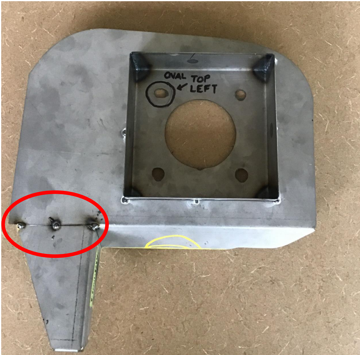
Orientate box as shown. Tack triangular corner piece to plate as shown
