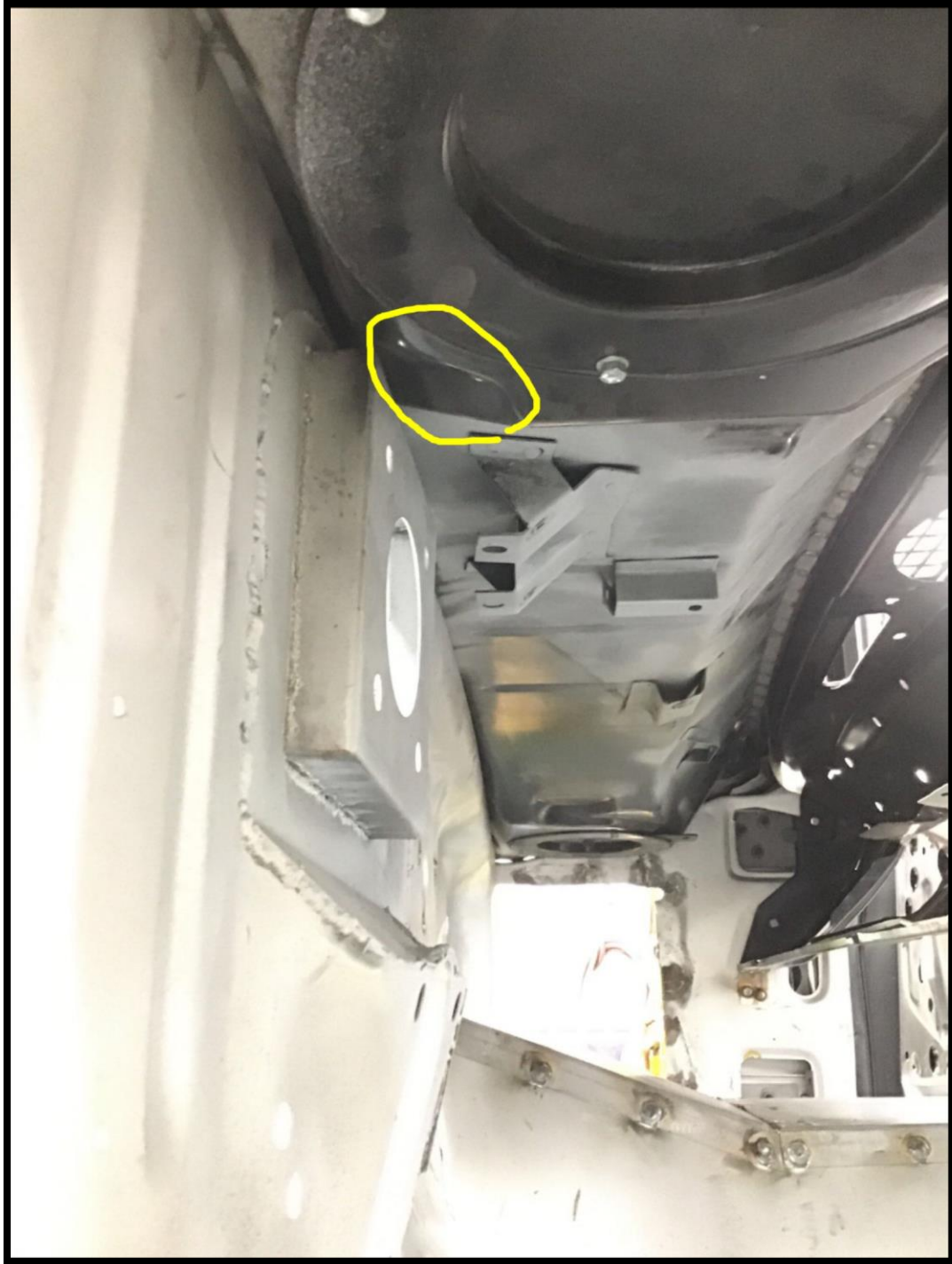
POUND COWL IN AS SHOWN TO CREATE CLEARANCE FOR PEDAL PACKAGE
