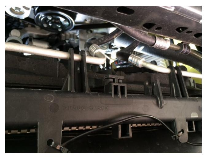
Step 4- Switch Installation. Run the single wire lead coming off the relay to the inside of the car. A good place to do this is right next to the brake booster thru the rubber grommet.
