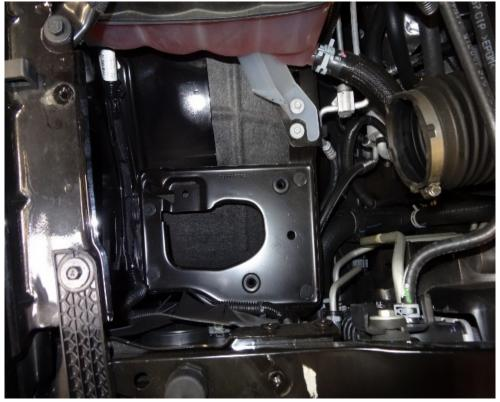
Step 2: :Disconnect the connector from the passenger side headlight. There may be a red, safety, tab on the connector. Remove the tab and then depress and pull the connectors off. Then install our harness inline with the headlight and the original truck harness.
