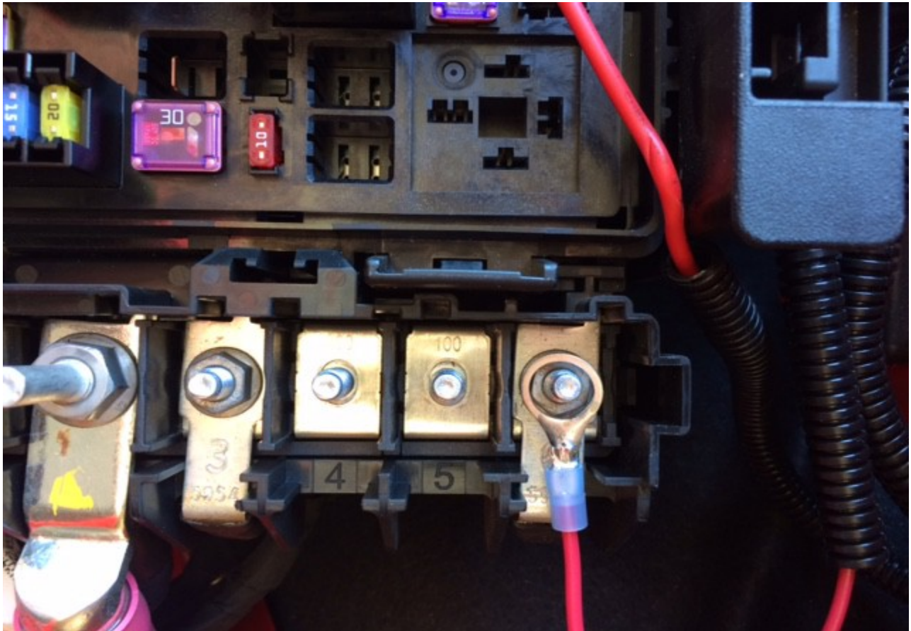
Step 9: Locate and remove fuse #50 from the under hood fuse block
