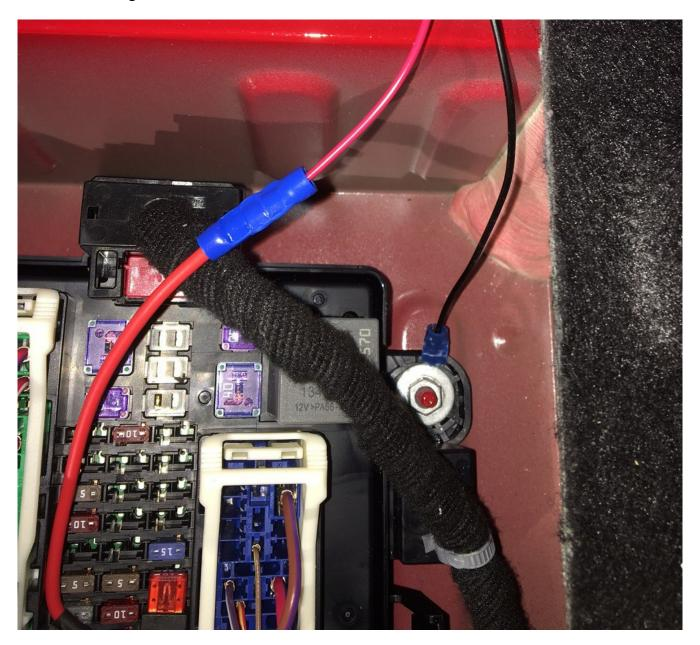
Step 19: Re-connect battery, start vehicle and test system. Once you hit the steering wheel heat button, the indicator on the wheel should illuminate and the wheel should then heat. Once operation is confirmed, reinstall all previously removed trim pieces and secure wires, under the dash, with tiestraps.
