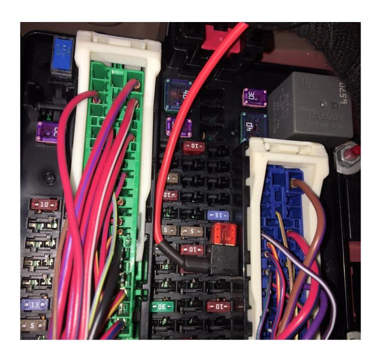
Step 18:Ground connection: Remove the 10mm nut from the side of the fuse block, install the ring terminal and re-tighten the nut.
