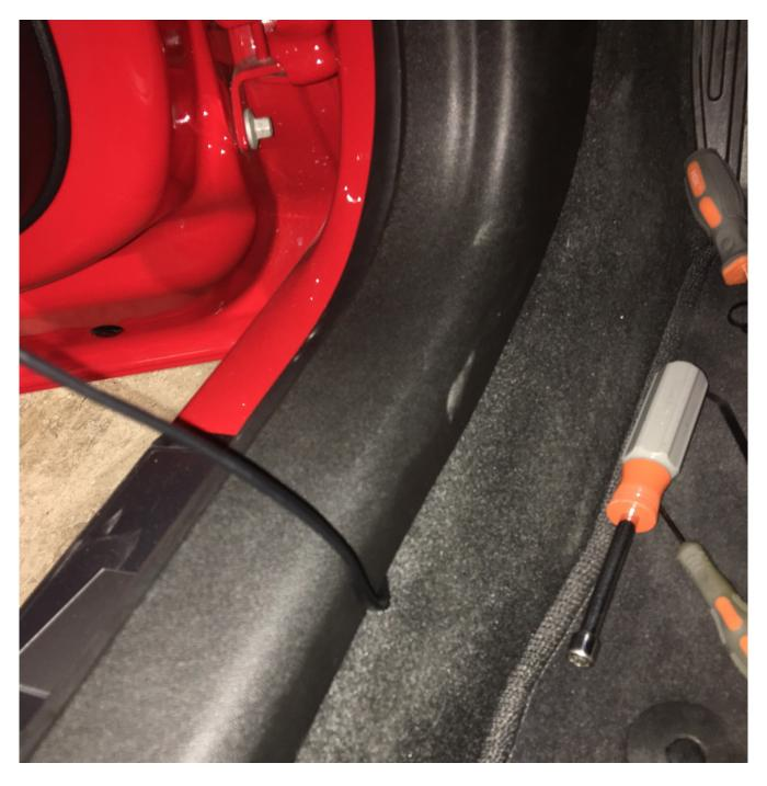
Continue tucking the wire along the rear quarter trim, position wire behind the seat belt anchor bolt. Once there you will want to push the wire up and behind the back seat so that the wire comes out into
