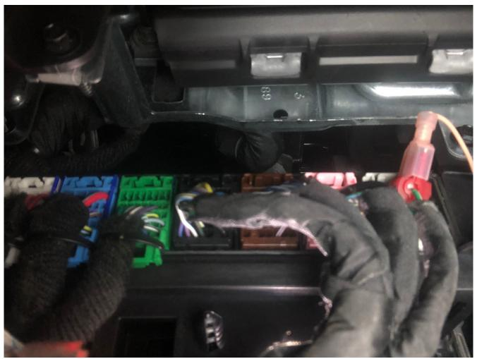
We will be working with the gray connector which is on the outside edge next to the pink connector. Unplug the gray connector and locate the green/white wire.
