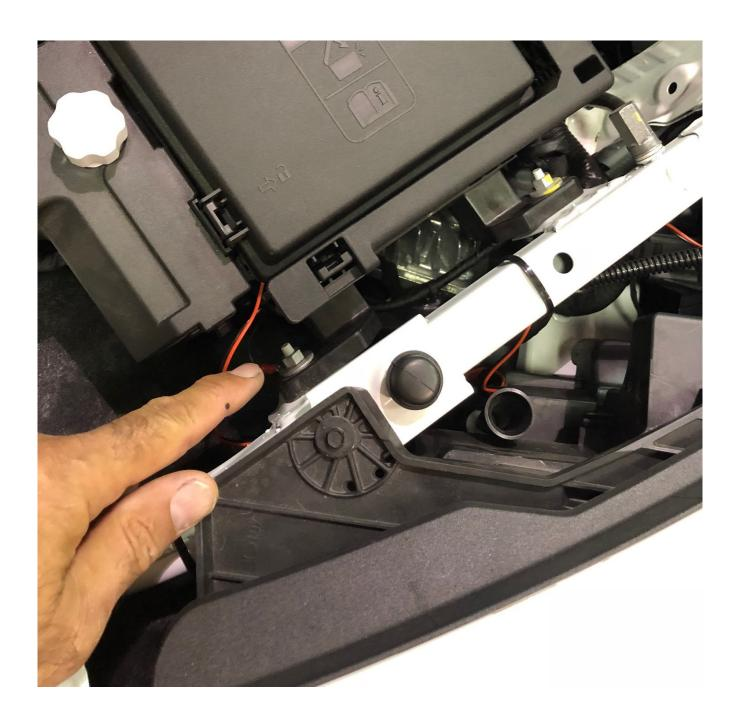
Step 4: Routing RCA cable into the inside of the car. Route the RCA along the inside of the fender toward the door area. You will then run the RCA cable around the felt.
