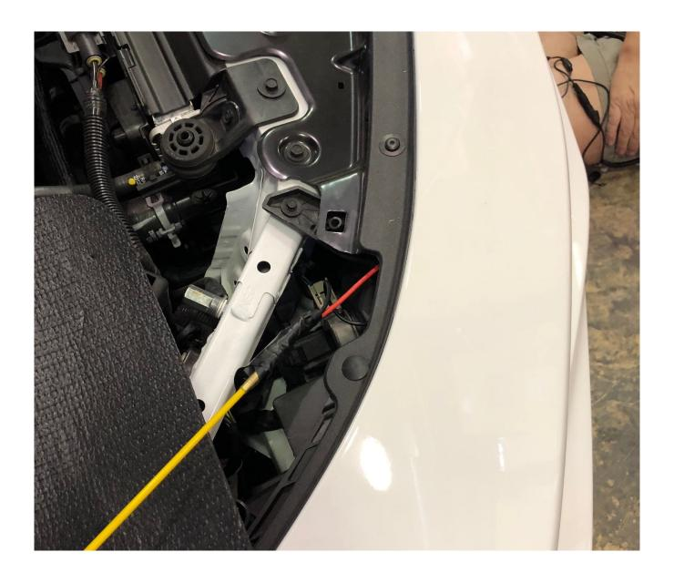
2-Mount lower camera to the lower grille area. You can either attach it with double sided tape or you can use, the included, clips to mount. You also could attach with screws, but you will have to remove the grille to do this. We have used both tape and the clips and have had excellent results.
