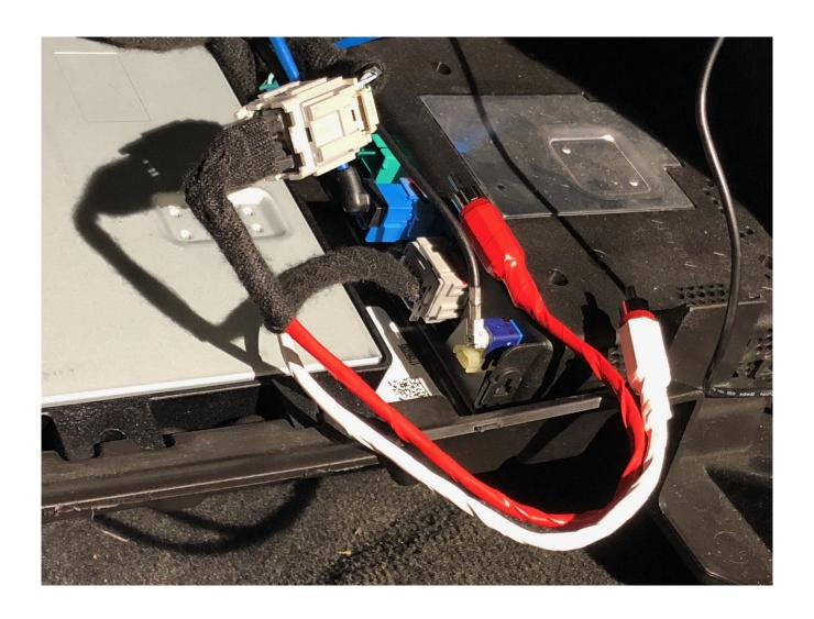
Step 6 :Once around the felt you can remove the body plug and poke a small hole in the plug. Then pass the rca thru the body plug and into the interior of the car. Simply pull the carpet back on the side to pass the cable thru.
