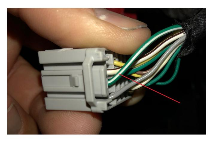
Install the supplied t-tap around this wire and slide the spade terminal into it. Please make sure that the center terminal of the spade goes into the t-tap. Once that is installed you can re-connect the gray connector to the BCM.
