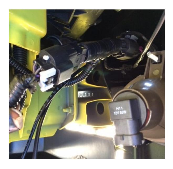
Step 3- Connect passenger side fog light harness to fog light and connect. Route driver's side of harness over and connect. Secure the harness to bottom side of radiator.
