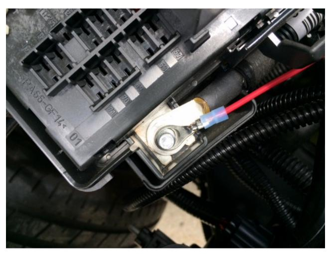
Step 2- Behind the passenger side of the bumper you will see where the bumper harness meets the body harness. Disconnect this harness and install, the Gen5DIY, harness inline.
