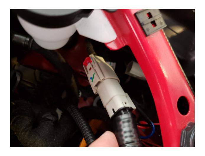
**Step 5**Take the other end of the Gen5DIY connector harness and now plug this into the headlamp directly
