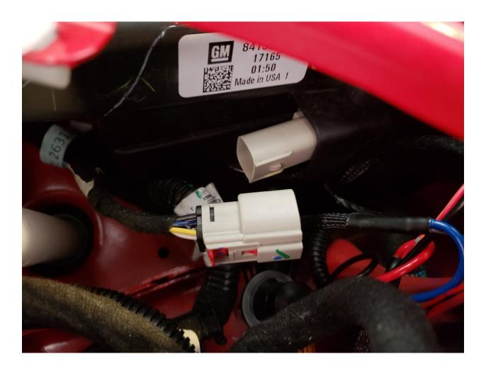
**Step 4**Take this end of the Gen5DIY harness and plug it into the connector you just unplugged from the headlamp. Ensure you hear it click and then slide the red locking mechanism down into place!
