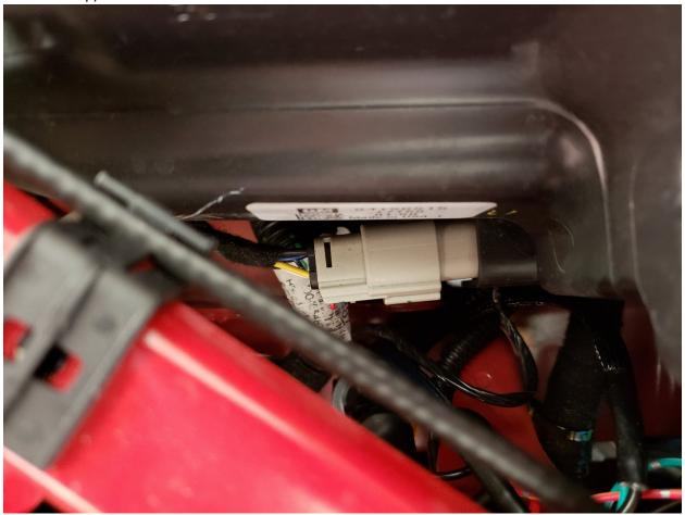
Using a pry tool or flathead screwdriver slide the red tap away from you and then push the tab in and slide connector away from headlamp housing
