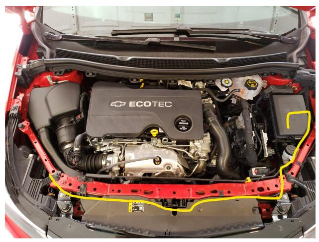
**Step 8**Locate the engine fuse box and remove cover
