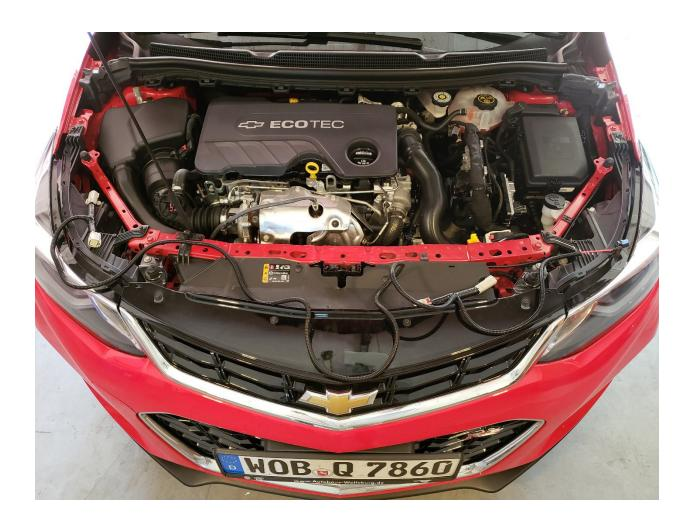
Locate the vehicle headlight plug pictured here for the dirvers side (looks the same for both right and left headlamp)
