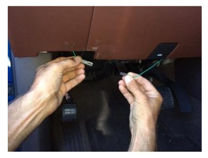
Step 16: Reinstall any remianing trim items. Start engine. On-star LED's should be lit, if on-star is activated you can try calling it for testing purposes.
