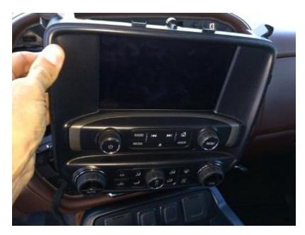
Step 12: On the backside of the screen you will notice a black connector that matches the otherr half of the Gen5DIY harness, unlplug this connector and install our harness inline
