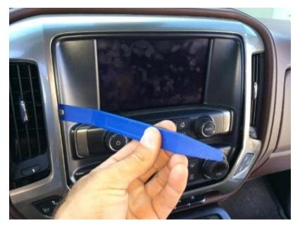
Step 11: Remove radio faceplate. Using 7 mm nut driver remove 4 screws
