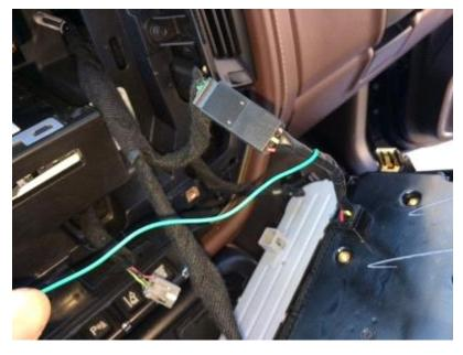
Step 13: Route green wire over to pocket and drop down behind driver's side knee bolster
