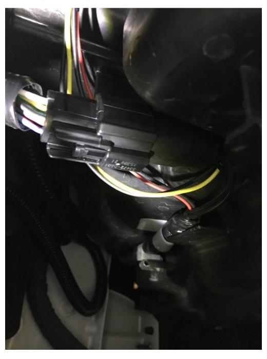
4- Route the passenger side of our harness over the top of the radiator and lower down to the passenger headlight. Plug this side inline.
