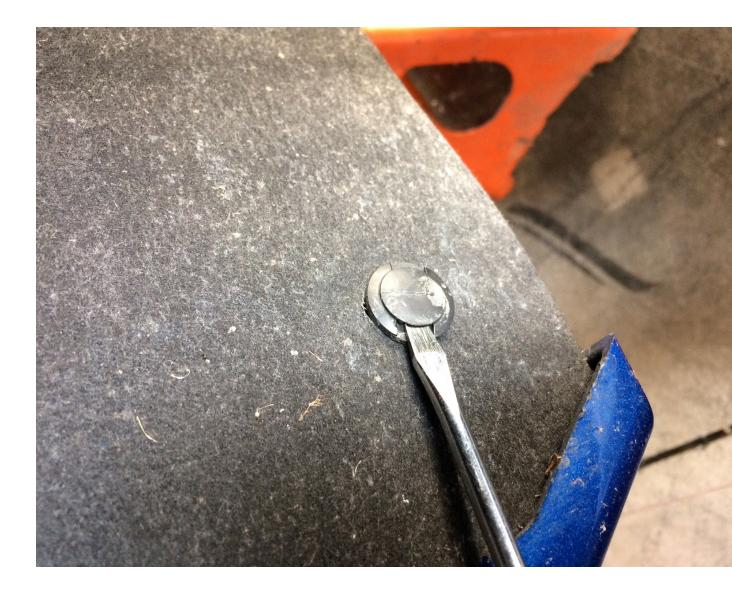
2- Remove 2 retainer clips from trunk liner with either a pair of side cutters or needle nose pliers. Remove carefully as to not destroy them.
