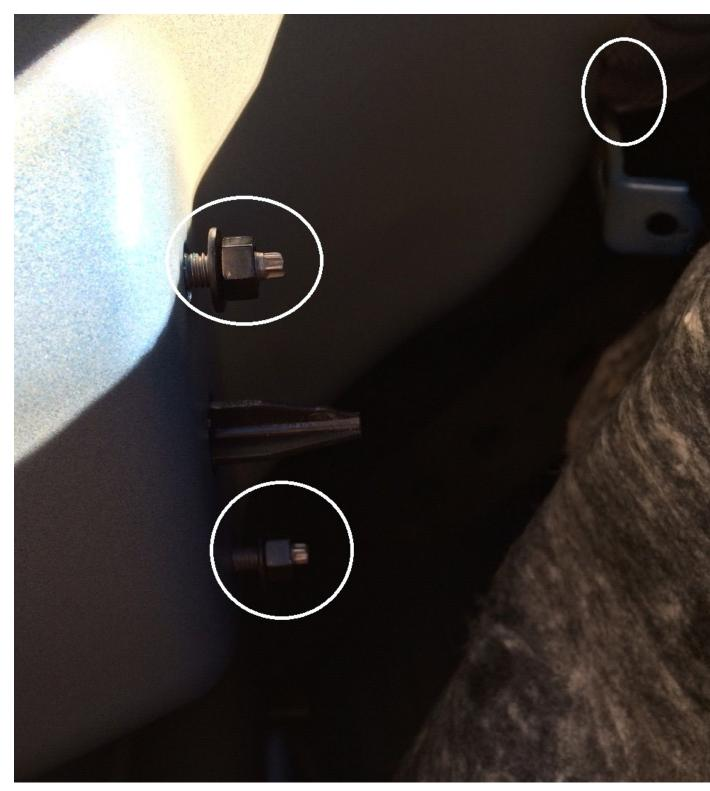
5: Once the nuts are removed you can remove the taillight by pulling back on the assembly. It does have guide pins so it may be a little snug. Be careful not to scratch your paint.
