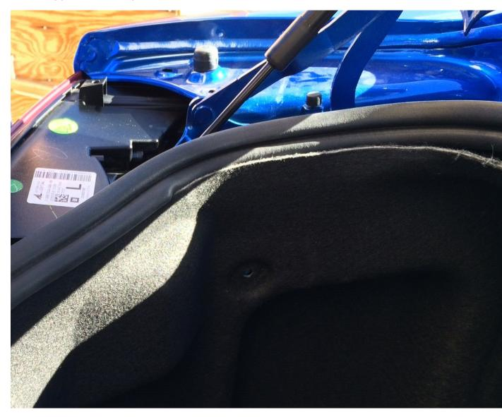
3- Carefully push down on top of liner and work out from under the truck seal.
