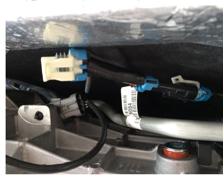
5- Plug other end of the Gen5DIY harness into the shift solenoid
