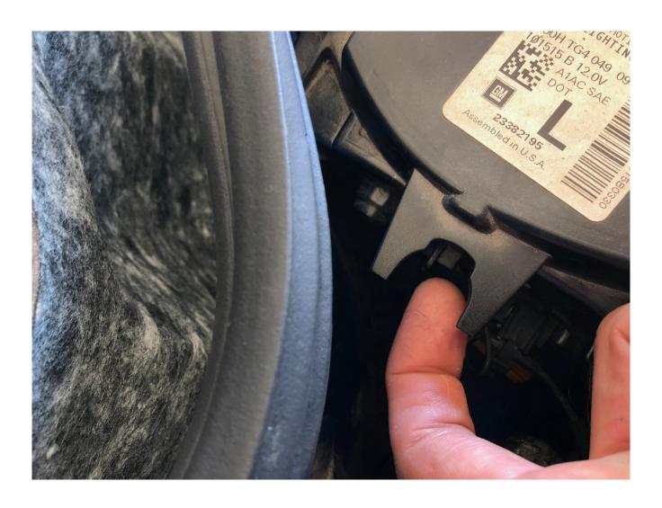
Step 4-Test for proper operation. LED bulbs are polarity sensitive, if one or both bulbs does not operate when you test please remove the LED bulb and rotate. In order to properly test the bulbs the engine must be running with the car in reverse. The reverse lights will not operate, in reverse, without the engine runni
