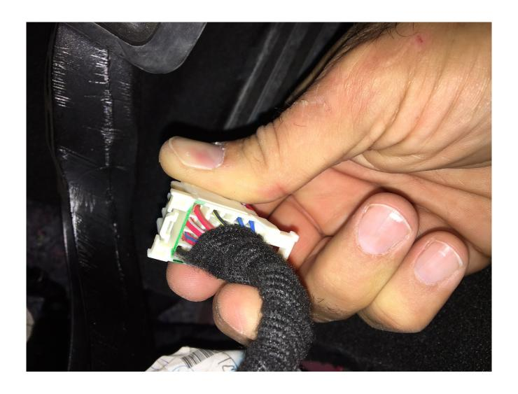
Step 15: Cut the tape back slightly to access the wires, about 2" is fine. Locate the white wire and attach the t-tap to it. Then slip the spade terminal onto the t-tap. Make sure that the terminal in the spade is centered so that it goes in correctly. Reinstall the BCM connector.
