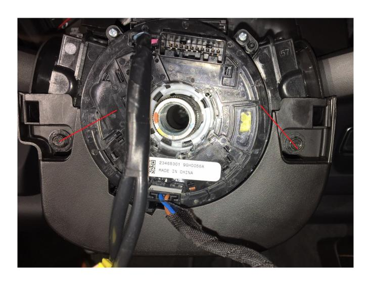
Step 5: Remove the clock spring by removing the 4 phillips screws and disconnecting the 2 harnesses on the rear of it and 1 harness on the bottom. You will have to remove the safety lock from the airbag connector to remove it.
