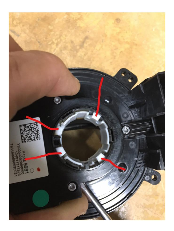
Step 7: Install single lead wire into the clock spring 10 pin connector. Remove the safety lock from the connector. Once removed insert the wire into pin # 4. You will hear a click when it is fully seated. Push the safety lock back into place.
