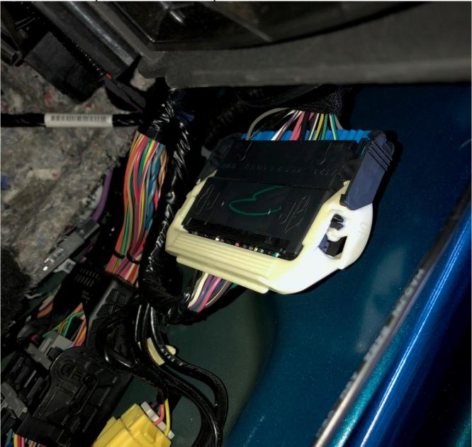
5- Locate the black wire located in A7. For reference A6 is brown/white and A8 is pink. Tie the loose black wire into the black wire in A7
