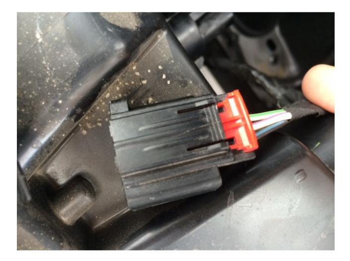
Step 3: On our harness the side with the fuse assembly is the passenger side. Plug the, Gen5DIY, harness inline with the original turn signal connector and the other end into the turn signal socket. Route the driver's side of the harness over to the driver's side headlight and connect inline as well. Secure the harness as needed.
