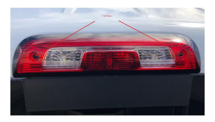
2- Pull brake lamp assembly out and disconnect main plug
