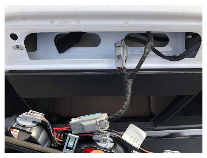
Step 4: Tuck harness into pocket and reinstall light.
