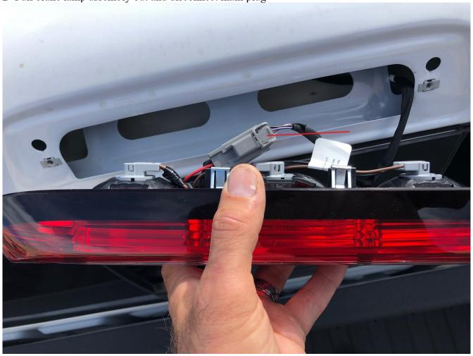
3- Connect the Gen5DIY harness to the brake lamp and into the original harness.
