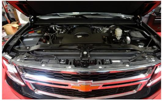
Step 2: Remove the air cleaner lid from the bottom lid and air intake tube
