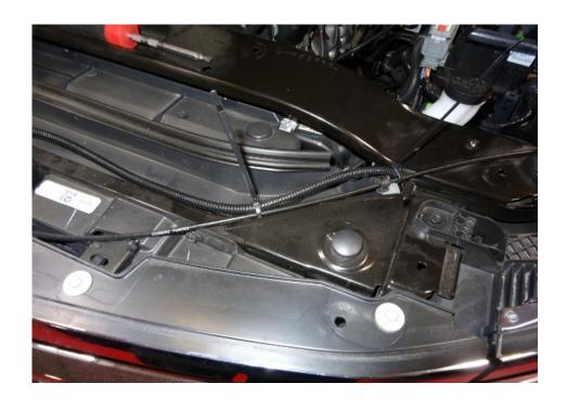
Step 6: Connect the Gen5DIY harness inline with each headlight and the original connector.
