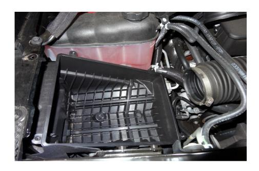
Step 3: Remove lower half of air cleaner by simply pulling up as it is held in with rubber grommets
