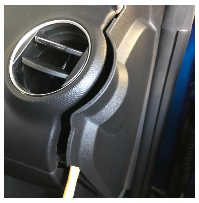
Remove inner sill plate by gently pulling out and up..
