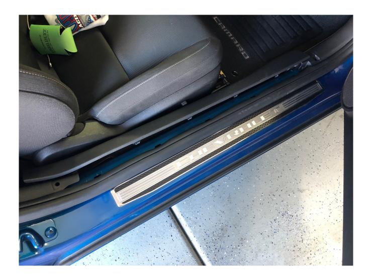
Remove side panel trim by releasing both the upper and lower trim clip.
