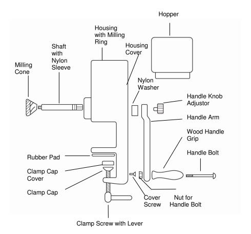
\*The handle arm, wood handle grip, handle bolt and nut for the handle bolt is considered the "Arm Assembly." These parts are not sold separately.
