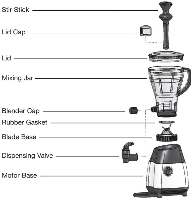
1. Position the rubber gasket down onto the circular flat surface in the blade base.
