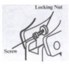
**SPECIAL NOTE:** This adjustment is only necessary for the mixing beaters and does not apply to the dough hooks, as they should not touch bottom of bowl during use.
