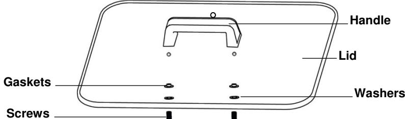
The hardware needed for attachment of the handle to the lid may be packed in a small plastic bag or within the handle itself. For glass lids, align the handle with the hole in the lid, and then secure with the screw assembly in the order shown above. **DO NOT** overtighten.
