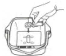
Do not use any abrasive scouring pads or cleansers on pan or knead bar as damage can occur. Wipe the inside of chamber and outside surfaces of machine with a soft damp cloth if necessary, dry with a soft cloth. **CAUTION:** To prevent personal injury or electric shock, do not immerse bread maker base, its cord or plug in water or other liquid.
