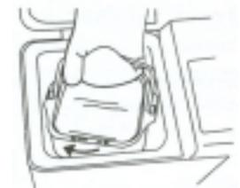
If bread is not removed when cycle completes, the bread maker will automatically go into **keep warm** for up to three (3) hours. The on light will remain lit and 0:00 will appear in display. When removing bread pan, always use oven mitts, as pan is still hot. Hold **start/stop** button down until on light goes out to turn bread maker off. Unplug cord from electrical outlet. If bread maker is not turned off during **keep warm**, it will automatically shut off after three (3) hours.
