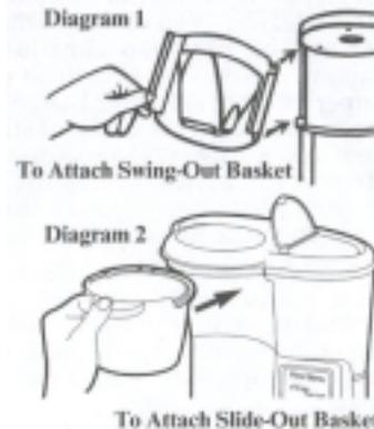
**Slide-Out Basket:** To remove basket, pull forward using handle. To attach basket, slide edge into guides at top until basket stops. See Diagram 2.
