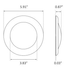
The Parmida LED Technologies™ 4 inch LED Disk Light is an industry shifting, truly ultra-thin light. The 0.03 inch thin Disk Light features as the ideal surface mount look, engineered for easy installation in any 2.75", 3.5" or 4" Junction Box. This product is built with Steady-Dim technology and is compatible with most modern LED dimmers.
