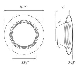
The Parmida LED Technologies™ 4 inch Baffle Design Downlight is an energy efficient take on a traditional retrofit light. This downlight is designed with an internal baffle trim to efficiently trap and shape the light downwards. Constructed with a durable metal trim, this product is built with Steady-Dim technology and is compatible with most modern dimmers, including Lutron Caseta Wireless systems.
