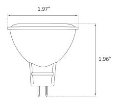
The Parmida LED Technologies™ LED MR16 is an enhanced and modernized spot light that will produce an even and focused light. Made with impact resistant, fire-rated polycarbonate material, this product is light, outstandingly tough and maintains it's original color over time. This product is built with Steady-Dim technology and is compatible with most modern dimmers.
