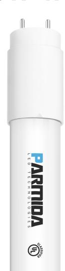
The Parmida LED Technologies™ 4FT LED Direct Wire Type B T8 tube can be installed by a simple bypass of the ballast. This tube can be installed with a single-ended or dual-ended connection and it can install directly into your fixture's original shunted sockets (tombstones), eliminating the need to retrofit your fixture with non-shunted sockets.
