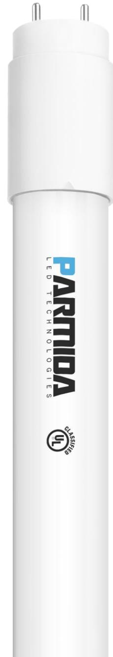
The Parmida LED Technologies™ 4FT LED Direct Wire Type B T8 tube can be installed by a simple bypass of the ballast. This tube can be installed with a single-ended or dual-ended connection and it can install directly into your fixture's original shunted sockets (tombstones), eliminating the need to retrofit your fixture with non-shunted sockets.
