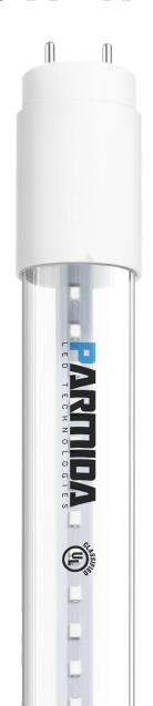
The Parmida LED Technologies™ 4FT LED Direct Wire Type B T8 tube can be installed by a simple bypass of the ballast. This tube can be installed with a single-ended or dual-ended connection and it can install directly into your fixture's original shunted sockets (tombstones), eliminating the need to retrofit your fixture with non-shunted sockets.
