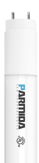
The Parmida LED Technologies 4FT LED Direct Wire Type B T8 tube can be installed by a simple bypass of the ballast. This tube can be installed with a single-ended or dual-ended connection and it can install directly into your fixture's original shunted sockets (tombstones), eliminating the need to retrofit your fixture with non-shunted sockets. These lights use only 24W to emit 3000 lumens (equivalent to 55W in fluorescent tubes), making them extra bright and energy efficient.
