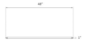
The Parmida LED Technologies™ 4 FT Type A+B LED T8 tube can function with or without a ballast. This tube can be installed with a single-ended or dual-ended connection. Fast and simple installation under the functionality of your choice, this tube is designed with user experience as the defining motivator.
