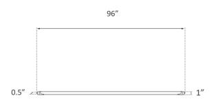
The Parmida LED Technologies™ 8FT 36W LED T8 Bypass Installation is a high-output energy efficient take on a traditional fluorescent 8ft tubes. These LED 8ft T8's are designed with a shatterproof lens which allows for safe installation in fixtures, with or without wire guards. This LED 8ft T8 requires a bypass installation with a dual ended connection and is compatible with FA8 Single Pin Base Fixtures.
