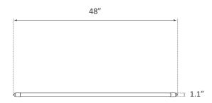
The Parmida LED Technologies™ 4FT LED Direct Wire Type B T8 tube can be installed by a simple bypass of the ballast. This tube can be installed with a single-ended or dual-ended connection and it can install directly into your fixture's original shunted sockets (tombstones), eliminating the need to retrofit your fixture with non-shunted sockets. Fast and simple installation under the functionality of your choice, this tube is designed with user experience as the defining motivator.
