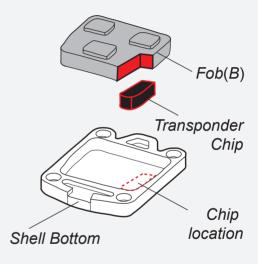
Note: To prevent rattling fill the gap between the Fob(B) and Transponder Chip with a piece of paper.
