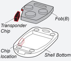
Note: To prevent rattling fill the gap between the *Fob*(*B*) and *Transponder Chip* with a piece of paper.
