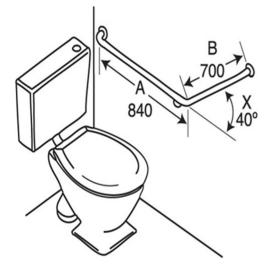
Finished Available 32mm Diameter Tube 32mm Diameter 1428 Knurled Mirror Polishing (No.9 Finish) Also Available in Powdercoated Colours
