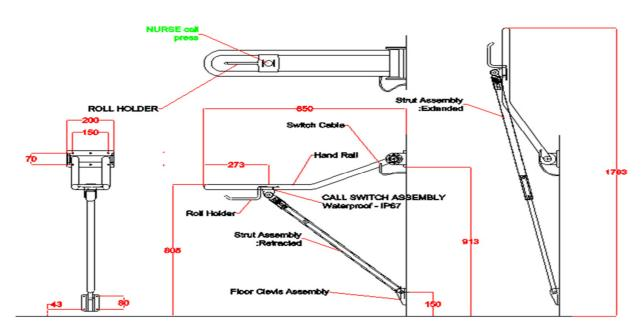
It is very important that a spacing block is utilised behind the rail to ensure that the rail is parallel to the wall surface as wall surfaces and squareness can vary. This can be adjusted on installation by an experienced tradesperson. The wall to the inside of the rail is 55mm on standard Bendtech Rails.
