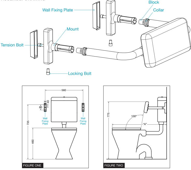
STEP ONE:Mount Wall Fixing Plates. Refer Figure One.STEP TWO:Establish Measurement "A". Refer Figure Two.STEP THREE:Cut tube to match measurement "A".<br/>(Line marked on underside of tube)STEP FOUR:Follow Assembly Drawing.
