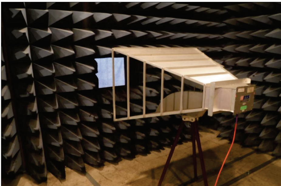
Photograph 2. Shielding Effectiveness, Big Horn EUT Measurement Receiver, Test Setup
