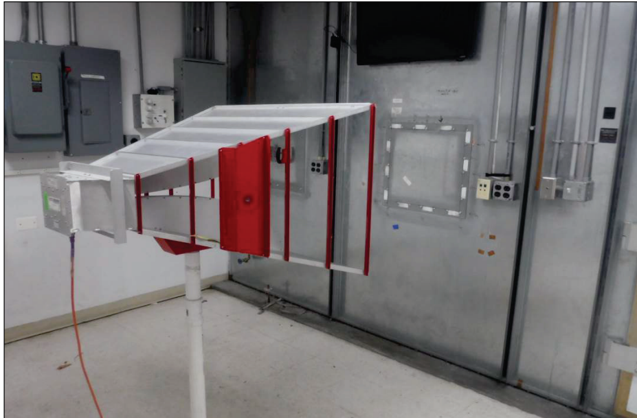
Photograph 5. Shielding Effectiveness, Big Horn Isolation Measurement Transmitter, Test Setup
