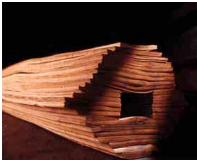
Veneer sliced and assembled in the shape of the log from which it came.
