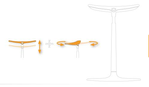
The comfort seat can be swivelled 20 degrees to both left and right. This creates flexibility and freedom, increasing the radius of operation, and so making it possible for the user to tackle every task in a dynamic way.
