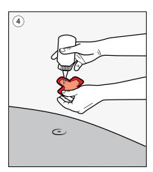
Always make sure that the patch you cut is larger than the area to be repaired. Apply super glue to underside of the patch. If you decide to repair the outside of your Fatboy® don't be afraid to have fun with shape of the patch, we encourage you to use your imagination.
