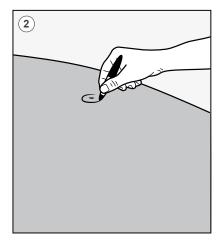
Identify source of leak. Define and mark the area to be repaired, repair can be made on the inside or outside.
