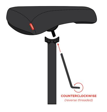
USE A STANDARD **5MM ALLEN KEY** OR ALLEN BIT TO INSTALL THE SEAT FROM THE UNDERSIDE. NOTE THAT THE BOLT TIGHTENS IN THE **COUNTERCLOCKWISE** DIRECTION. STEALTH SEAT + PIVOTAL SEAT POST
