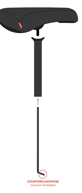
IF YOU DO NOT HAVE A STEALTH SEAT POST, A STEALTH SEAT MAY BE INSTALLED WITH A TRADITIONAL PIVOTAL SEAT POST BY USING AN EXTRA-LONG ALLEN KEY INSERT THE EXTRA-LONG **5MM ALLEN KEY** UP THROUGH THE SEAT POST, UNTIL IT EXTENDS OUT OF THE TOP OF THE POST. NOTE THAT THE BOLT TIGHTENS IN THE **COUNTERCLOCKWISE** DIRECTION.
